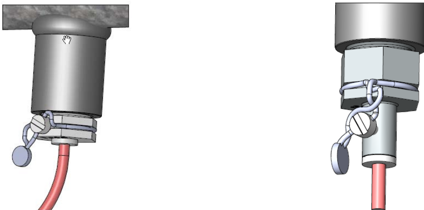
Figure 25: A number of examples of sealing of temperature sensors, either with sealing wire or sealing shells.
