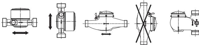
2. For water meters no inlet and outlet distances must be adhered to.
