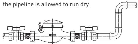
11. With many installations water pipelines serve as earthing for electrical systems. Depending on the actual application an electrical bypass of the water meter is to be ensured.
