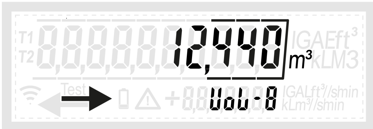
Figure 20: Exemplary screenshot of back flow volume register as shown in display sequence
