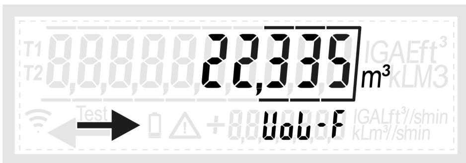
Fig. 21: Exemplary screenshot of forward flow volume register as shown in display sequence
