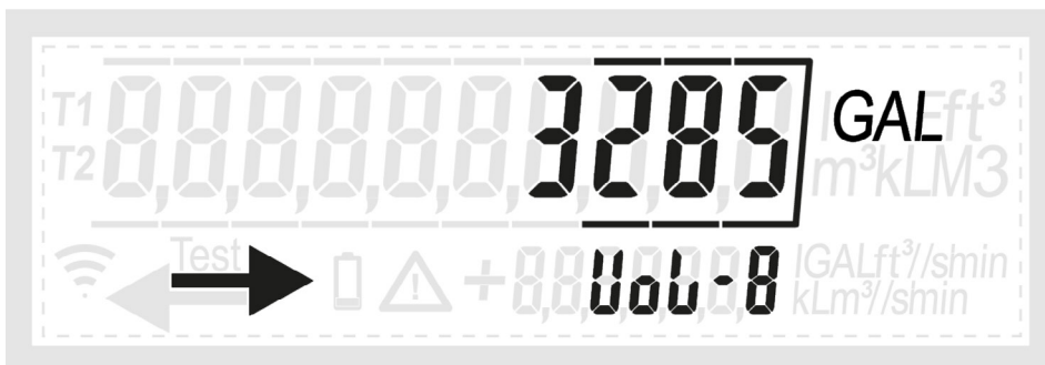
Fig. 22: Exemplary screenshot of back flow volume register as shown in display sequence
